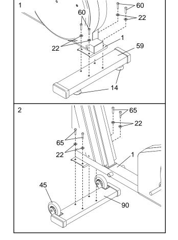
2. Attach the Front Stabilizer (90) to the Frame (1) with the four M10 x 43mm Screws (65) and four M10 Split Washers (22). Make sure that the Front Stabilizer is turned so the Wheels (45) are not touching the floor.
